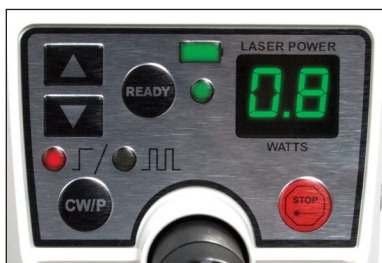
Sapphire Plus STM 3W Diode Laser control panel showing that the laser working beam is emitting in CW at 0.8 W.
