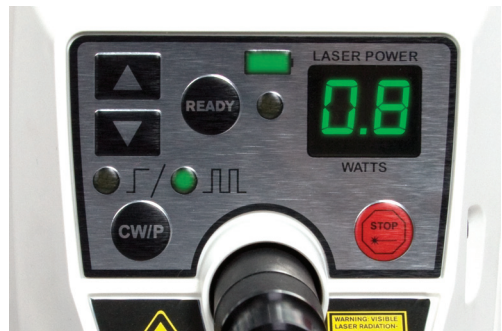
STAND-BY, P Mode 0.8W output
