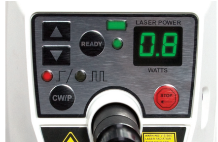
Saphire® Plus STM control panel showing that the laser is emitting in CW at 0.8 W
