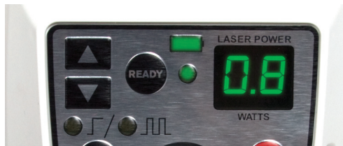
Laser in READY Mode @ 0.8W output
